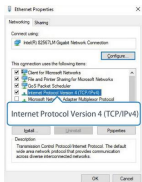
⑤. Double Click "Internet Protocol Version 4 (TCP/IPv4)" to configure IP address and DNS server.
