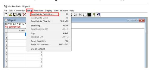
Set the default slave ID(7-in-1 is 20), function code 04, starting address 0, quantity (7-in-1 is 28);
