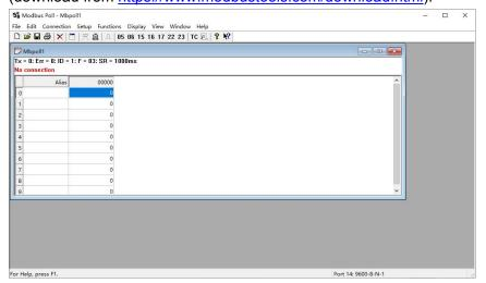
Configuration connection parameters: Baud rate 9600bps, 8 Data bits, None Parity, 1 Stop bits.
