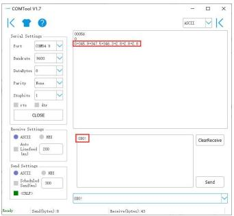
Then send "continuous measurement command 0R2!, the device returns 4 measured values: cumulative rainfall 1.2mm, cumulative rainfall duration 20 seconds, rainfall intensity 1.2mm/h, maximum rainfall intensity 72.0mm/h.
