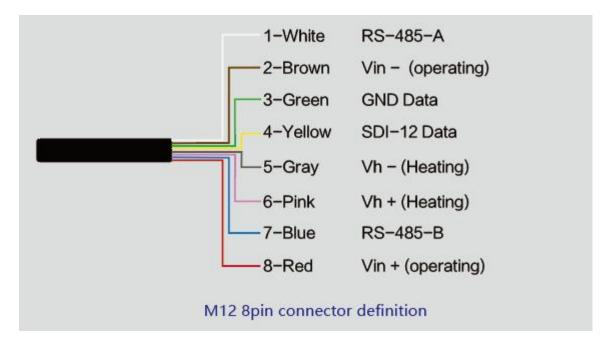
The device adopts an M12 8-pin connector, the different colored pins provide power and data communication (as shown in the above diagram).
