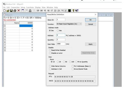
Now the computer reads the sensor data every 1 second, and the measurement (line 0 and line 1) is shown in below picture, after dividing the measurement by 1000, it is the true temperature value,  $28300/1000 = 28.3 \,^{\circ}\text{C}$
