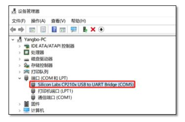
If the driver is not installed automatically, click this link to manually download and install the driver. (The
