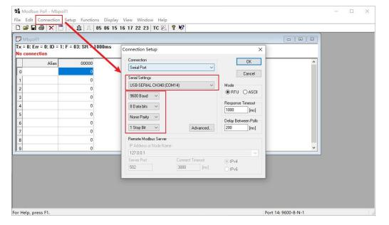
Read the air temperature register 0x0000 to 0x0001, click Setup, and select Read/Write Definition
