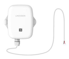
S500DI is a compact LoRaWAN® pulse counter which transforms traditional water meters into wireless intelligent meters. With IP67 waterproof design, it is applicable in various harsh application environments.
